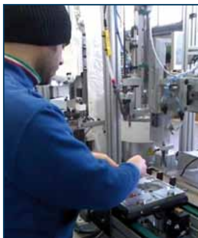
Example of system with electric nutrunner motor integrated into production lines
