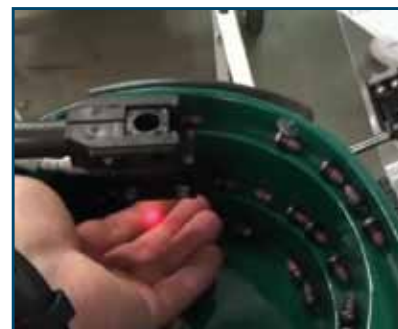
Screw feeder with 'over-unloaded' sensor for activation of screw feed (upon request)
