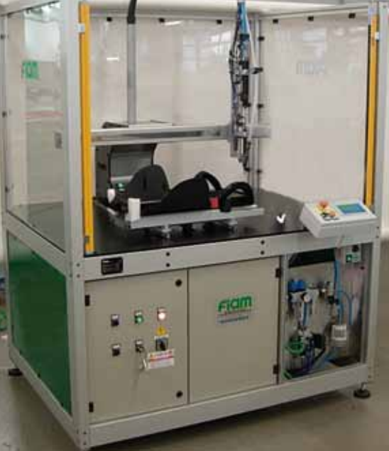
Example of EasyDriver MCA integrated on pre-existing machine with electrical cartesian axis X, Y
