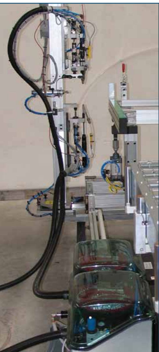
Example of multiple EasyDriver MCA for shutters field: assembly from the top towards the bottom and from bottom towards the top
